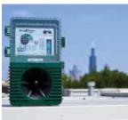
The BirdXPeller PRO is a sonic bird repeller that broadcasts a variety of naturally recorded bird distress signals and predator calls that frighten, confuse and disorient pest birds within the effective range. Pest birds cause damage, liability and health hazards. Sonic bird control is a safe, humane, eco-friendly way to get rid of birds from outdoor areas. Sonic repellers use high-definition recordings. digital Customizable
