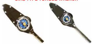
Dial Type Wrenches provide unmatched reliability, accuracy and durability for applications where torque measurement is extremently critical. Models feature a memory pointer that indicates the highest torque achieved during application of torque. 2% accuracy clockwise and counterclockwise. All wrenches are made in the USA of all steel construction for the highest quality. Both models come with a plastic storage box and a calibration compliance certificate.
