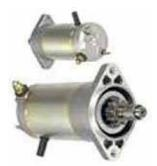
(Replaces Rotax P/N 995-430) Voltage: 12 kW: 0.6 Condition: New Rotation: CW Starter Type: PMDD Number of Teeth: 9 Gear OD: 1.154" / 29.3mm Mtg Ear 1 Hole: M8-1.25 Threaded Mtg Ear 2 Hole: M8-1.25 Threaded Weight: 5.2 lbs / 2.36 kg.
