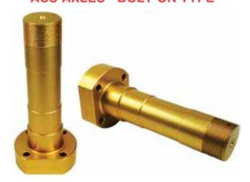
500X5 AXLE - Machined from 2024T3 aluminum. Gold anodized per specification MIL-A-8625C, Type II for improved corrosion resistance. Length 5-3/4". Mounting bolt pattern is four equally spaced 1/4" dia. holes on 1-15/16" dia. bolt circle. Thread size: 1-1/4 x 16.
