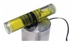
This extremely simple and sensitive tool uses the plum-bob and bevel principle to balance props both vertically and horizontally. It can be carried in a small tool box for easy use in the field and balances props accurately for smooth operation. The precision machined hub works with any prop designed with standard 1" center hole. Illustrated instructions .....P/N 13-17400 ......\$29.95
