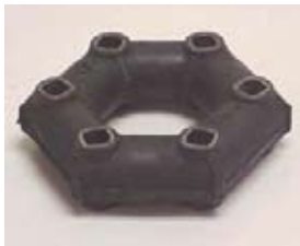
Photo # 3 – The Rubber Hardy Disc protects the crankshaft from shock loads. Check thru large inspection holes in side of model “C” & “E” gearboxes for possible tearing.
