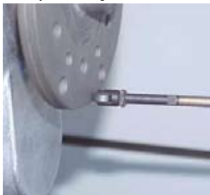
Photo #1 – Check the prop Flange for run out. Maximum of .003" is allowable.
