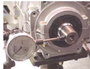
Photo #2 – Check crankshaft at end of taper as shown with roller tipped dial indicator.
