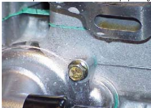
Photo #5 – Pressurizing the system to +5 psi and spraying the block with a solution of 50% water and 50% liquid dishwashing soap will pinpoint any leak. Here we have loosen a water pump housing bolt during the cooling system test to show the bubbles created by a leak.
