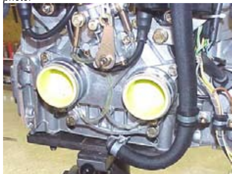
Photo #3 – Plugging the intake manifolds is easy with these tapered plastic plugs. CPS Part # 9734.
