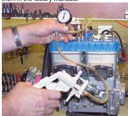
Photo #1 – With the use of a few plug caps, hand pump and gauge. We can test both the combustion chamber and the cooling system for leaks and possible trouble.
