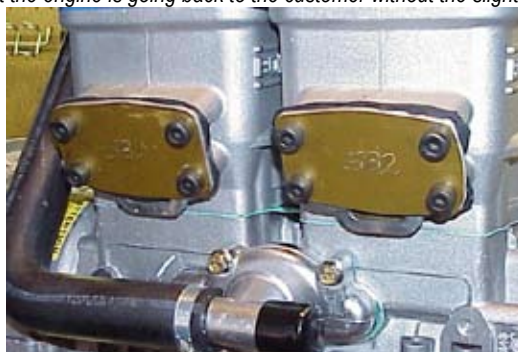
Photo #2 – Sealing the exhaust ports with 1/8" thick aluminum plates and rubber gaskets will allow us to pinpoint possible leaks in the combustion system.
