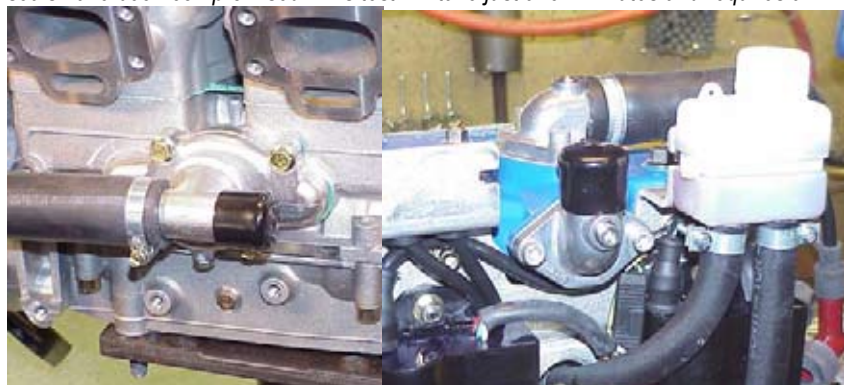
Photo #6 – Capping the water outlets is easy with these 1" rubber caps Part # 9723.
