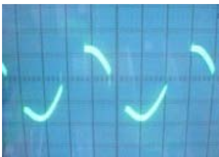
Figure #11 – KW Blue Box Regulator with 2-amp load on DC side. 2 volts per Div. *
