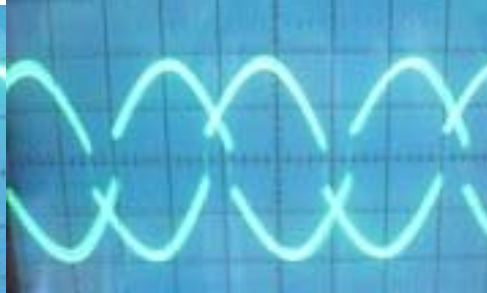
Figure #10 – KW Blue Box Regulator with no load on DC side. 20 volts per Div. *
