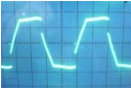
Figure #13 – KE Precision Power Supply with a 2 amp load on its DC side. 20 volts per Div*
