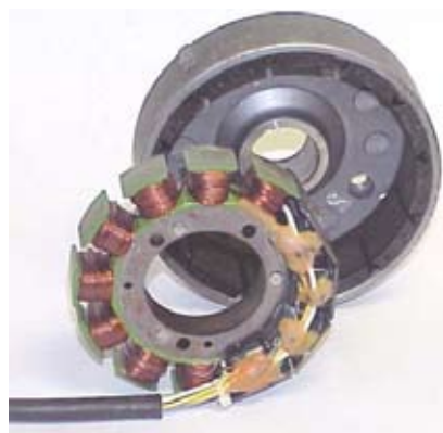
Figure #1 – The heart of the Ducati Magneto Generator. Note the four windings dedicated to the ignition and the 8 poles dedicated to the alternator.
