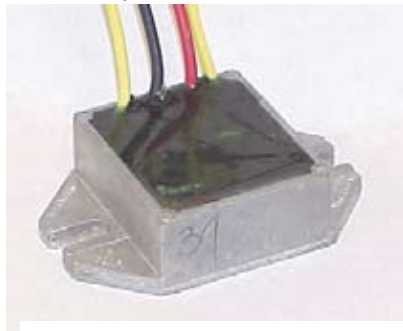
Figure #3 - This #9103 or Rotax #866-080 regulator is the simplest and cheapest regulator on the market. Sells for around $30.
