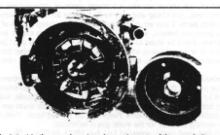
Photo 2: A look inside the mag housing shows the guts of the new Italian-made dual ignition. A 12 coil "radial" type layout provides 175-watt output as well as dual spark plug voltage; 180-degree opposed trigger assemblies are recessed into the mag housing; and two rotating flywheel magnets signal spark timing. There is no timing adjustment to set!
