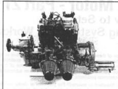
Photo 4: A side view shows the new gear box mounting. No adapters. All new production engines use this simplified and versatile system.
