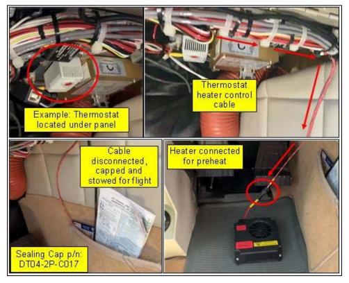
**Figure 7.13.** Example Occasional use heater. Cabling and thermostat permanently installed with lead for heater positioned clear of controls for connection with heater during preheat. Refer to Thermostat Instruction: TN03235, §§ 4.9 and 4.10.
