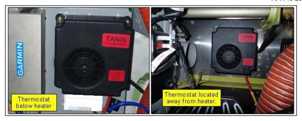
**Figure 7.5.** Examples of AV heater installations.
