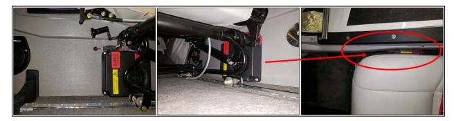
**Figure 7.7.** PA-28 example w/ heater on sidewall below door sill. Installation used existing firewall passthrough for cabling routing from engine preheat power plug. Thermostat remotely located under avionics panel, refer to instruction TN03235.
