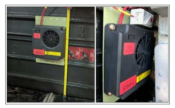
**Figure 7.9.** Helicopter installation, example w/ heater located on bulkhead with field fabricated mounting plate/bracket drawing 03331. Riveted to longerons with CR3212-4 blind rivets. Thermostat mounted on plate above heater, refer to instruction TN03235.
