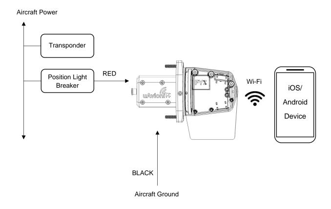
WARNING: Do not connect the power wire to a Xenon strobe power pack. This can damage the light and voids the warranty.
