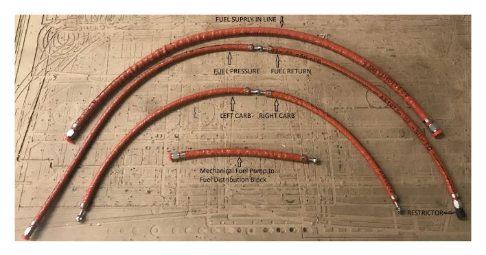
In addition to the restrictor fitting, we also include the Adapter fittings for your fuel pump in and out fittings.
