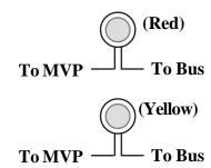
B. Mark the aircraft instrument panel and drill a 5/16" hole for each light. Install the Red Warning Light and the Yellow Caution Light from behind the aircraft instrument panel.
