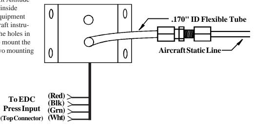
4" flare union. Care should be taken not to put excess pressure on the flexible line. <u>Make sure the flexible line does not kink.</u>
