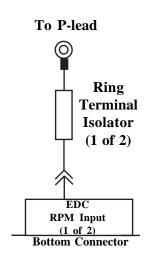
**WARANING:** Connecting an EDC RPM input directly to a magneto without an Isolator will damage the EDC. Be sure there is an Isolator in each RPM input lead connected to a magneto, ignition coil or CDI ignition.
