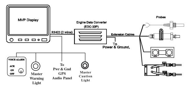
The MVP-50P (MVP) display measures 5.55" wide by 5.15" high by 2.4" deep and is designed to be mounted from behind the aircraft instrument panel. The MVP could be mounted onto a sub-panel which would then be mounted to the aircraft instrument panel from the front. The installation location of the MVP display on the aircraft panel and the method used to install the display will be a primary consideration in your decision to install the MVP.
