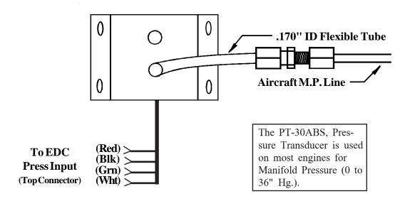
Connect the aircraft manifold pressure line to the pressure port on the PT-30ABS Pressure Transducer. Be sure this line is tight. This pressure port is a 1/4" flare union and is standard for most manifold pressure lines. Care should be taken not to put excess pressure on the flexible line between the flare union and the pressure transducer. Make sure there are no kinks in the flexible pressure line.
