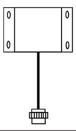
To EDC Resistive Fuel Level Inputs (Bottom Connector) and the Fuel Level Sensor.
