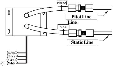
the PT-05Diff. Be sure these lines are tight. The ports are 1/4" flare union. Care should be taken not to put excess pressure on the flexible lines. **Make sure the flexible lines do not kink.**
