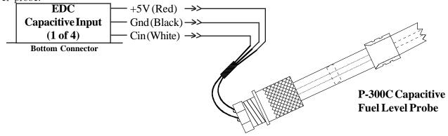
Note: The capacitive fuel level channels are shared with the resistive channels. A single capacitive and resistive channel cannot be used simultaneously.
