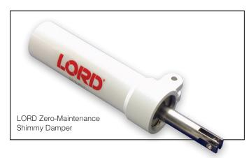
The LORD® fluid-free shimmy damper offers high-performance damping and vibration control with a zero-maintenance design. It uses surface-effect technology to provide consistent damping for fixed and retractable landing nose gears. Instead of using fluids to resist motion, the shimmy damper features a unique elastomer formulation to absorb nose wheel shimmy. Since there is no fluid, this damper will never leak.
