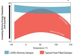
LORD surface-effect dampers operate consistently in the -40° to 150° Fahrenheit range while traditional hydraulic dampers only provide peak energy dissipation in the 20° to 80° Fahrenheit temperature range.
