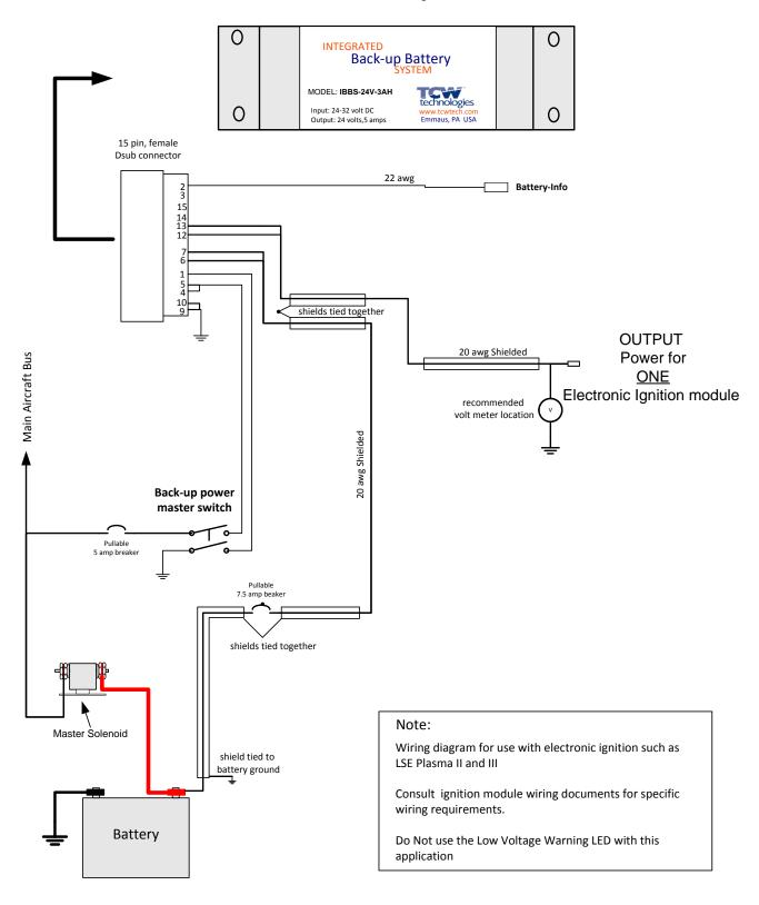
Advanced Flight Systems 5000 series wiring
