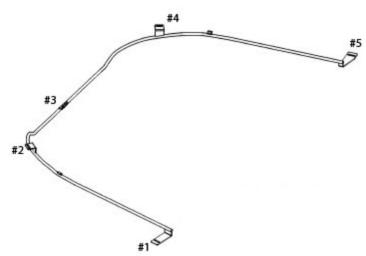
The Hawker Monorail Sunvisor System is designed to bolt into your aircraft without drilling any holes or installing specialty fastening devices. There have been a few aircraft where rivnuts or nut plates will be required and we have added 2 A10K80 rivnuts just in case this is the case in your aircraft.
