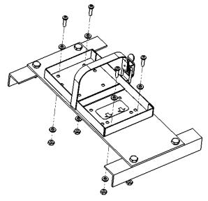
Figure 13 Typical Mounting Tray Installation
