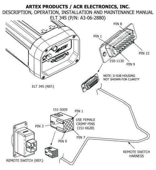
Figure 19 Remote Switch Harness Arrangement
