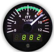
Electronics International Inc. will configure the TR-1-ITT to the range limits based on the data provided by the pilot/owner and/or mechanic. The data must match your aircraft's POH/AFM and all changes required by AD's, Supplements and/or STC's. Also, limits may be crosschecked against the instrument previously mounted in the aircraft panel. If any of the information provided on this form is wrong, there will be a fee to change the configuration.
