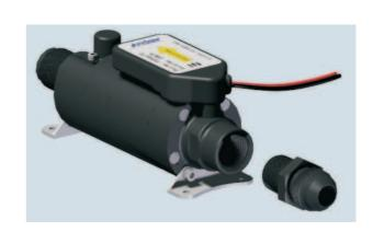
Within the body of the Boost Pump is contained the Bypass. This feature allows for fuel to flow around the positive displacement pump, whilst the pump is not running. The porting within the body has been computer optimised to ensure the best possible flow conditions.
