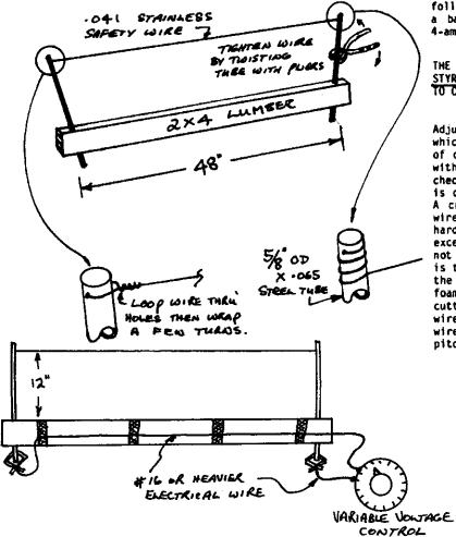
The Variable voltage control can be obtained from a Solitaire distributor or you can substitute any controllable power supply to include the 14 to 20 volt range with at least 4 amp capability. An alternative is to borrow two 12-volt battery chargers or auto batteries and lash up the following device. The "A" blocks represent either a battery or a 12-volt DC battery charger with 4-amp capability.
