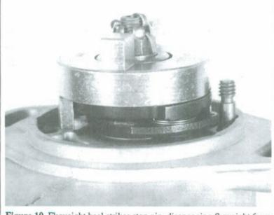
Figure 19. Flyweight heel strikes stop pin, disengaging flyweight from stop pin. Impulse coupling spring spins magneto.
