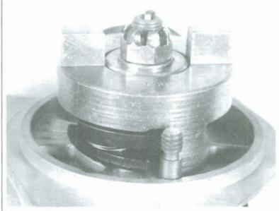
Figure 18. Impulse coupling as installed on magneto. Start position with flyweight toe engaged against stop pin. Magneto is prevented from turning. Impulse coupling spring winds up.
