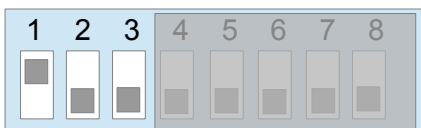
Node address 2, breakers 9-16
