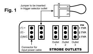
TYPICAL STROBE HOOK-UP PIN 1 - RED - ANODE PIN 2 - BLACK - CATHODE PIN 3 - WHITE - TRIGGER
