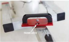
Attach to your airplane by holding both handles for alignment and then twist the attachment handle to lock it onto the lugs. Make sure the thumb latch has engaged so there is no chance it will accidentally come loose during use.
