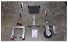
Unpack and inspect components: Tow Arm, Operator Platform, Handle Bars. Drive Head, 5/16-18 x 7/8 Hex Bolts (10)
