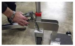
Every month or as needed apply 2 pumps of grease to the grease fitting on the drive head as shown. Also from time to time apply a light coating of grease to the outside of the lug tubes and the diagonal slot on the tow arm.
