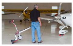
Transport the GoTow to and from your airplane by either carrying it or using the transport wheels as shown.
