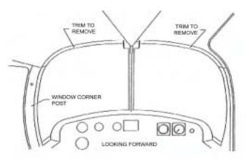
towards the rear of the aircraft. The mounting bracket should be above and inboard of the trim piece on the window corner post. Mark both mounting holes.
