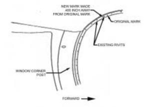
Eugene, Oregon USA 97405 www.rosenvlsor.com 541.747.0034 Page 1 of 2 • Measure to the rear of the forward metal lip where you just marked the outboard hole .40" and verify that when the visor is held up to this position the end of the lens is not across the centerline of the aircraft. The mark should not be on any existing rivets but between or beside one of them.
