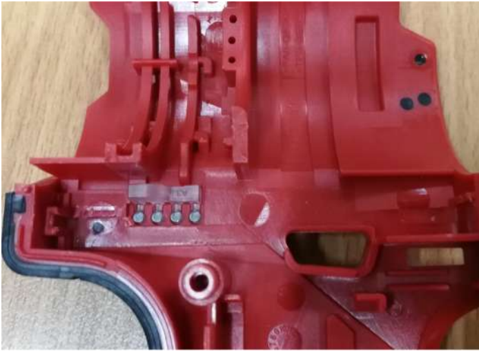
STEP 1: Insert light pipe in cavity of left housing halve-support.
