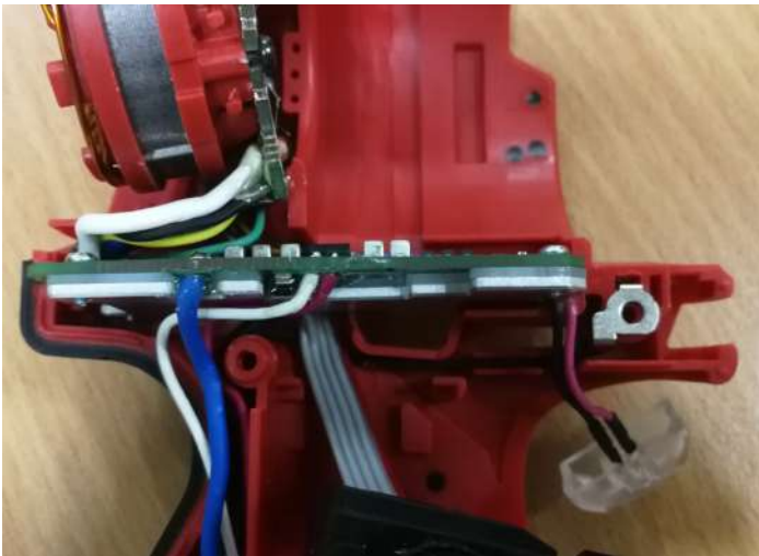
STEP 3: Assemble PCBA into corresponding housing cavity as shown.
