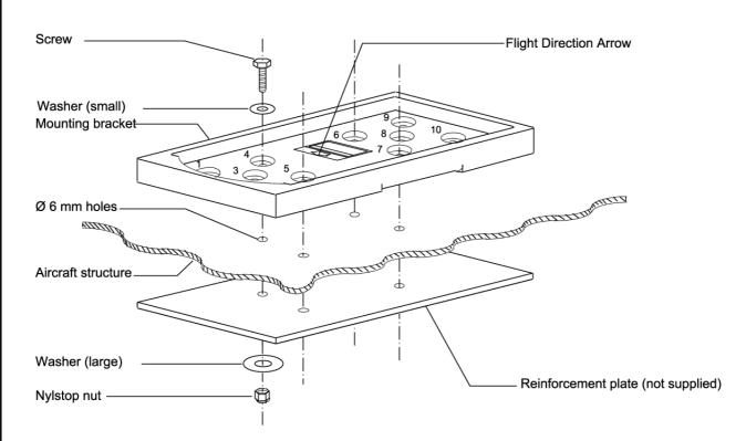
Figure 3: Bracket installation
