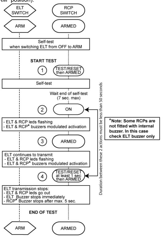
Figure 301: RCP LED and buzzer operation
