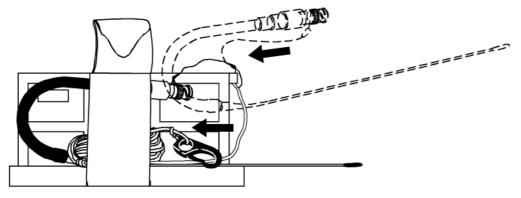
Connect the external antenna to the BNC connector (Refer to Figure 5:
