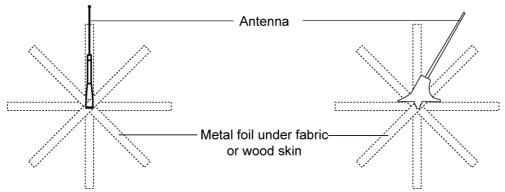
Figure 6: Antenna ground plane for non metallic aircraft
