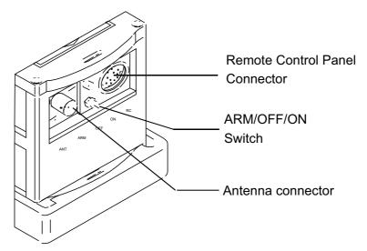
Figure 5: Installation, controls and connectors
