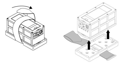
Figure 7: Removing the transmitter
