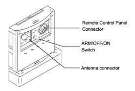
To operate the ELT with the Remote Control Panel, ensure that:
