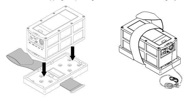
Figure 204:Installing the transmitter on the bracket
