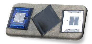
The Adhesive Epoxy Pads are a non toxic, zero V.O.C., performance thermoplastic adhesive designed to adhere raised pavement markers to the concrete or asphalt surface. When heated with a propane heat torch, a Pad liquefies and fuses with the surface and the marker providing a bond that will last throughout the marker's lifetime.
