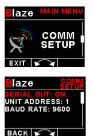
**Serial Out:** Select "ON" to enable the RS232 serial output.
