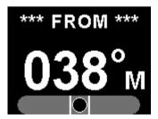
Press the F2 key to activate the reverse course display. This display remains active for about 5 seconds before reverting back to the normal heading display.
