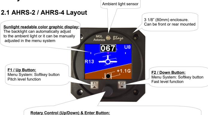
Press the rotary control during the normal display screens to access the menu system. Rotate anti/clockwise for up/down menu scrolling. During normal mode turning the rotary control anti/clockwise will scroll through the main displays (Artificial horizon, compass and turn and bank indicator).
