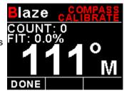
Fly a number of banked 180 or 360 degree turns at different bank angles - i.e. shallow, medium and steep turns. Try to add many different pitch attitudes in various orientations relative to the field direction. It does not matter in what order you fly the maneuvers. A typical, good calibration tends to take 5-10 minutes of flight.
