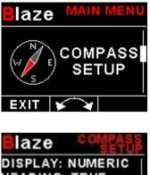
DISPLAY: NUMERIC HEADING: TRUE MAG VAR: MANUAL VARIATION: 0°E FILTER: MEDIUM SLIP: ON SLIP SENSE: LOW SLIP ZERO CAN ADDRESS: 1 CALIBRATE BACK
