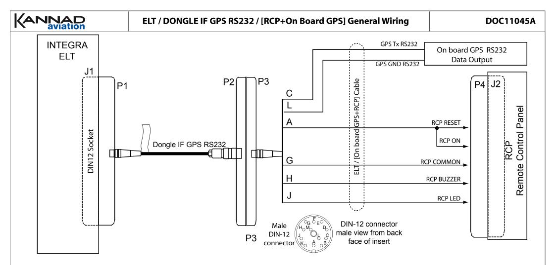
Fabricate a 6-wire AWG24 shielded bundle long enough to reach between the ELT installation location and the cockpit panel RCP and GPS equipment location.
