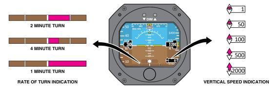
Figure 4.2, Rate of Turn & Vertical Speed Indication
