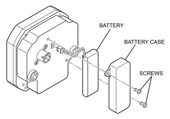
Figure 4.7, Battery Replacement
