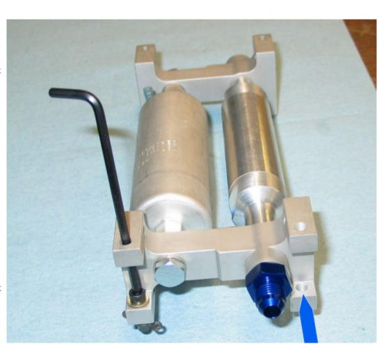
Pump Module. In the photo, the washer on the right has been trimmed a bit on one side to provide clearance with the manifold portion of the Boost Pump. The washer on the left side does not require the trim do to the shape of the manifold.
