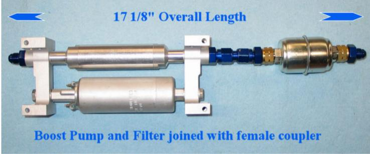
of 17 1/8". In some cases it is desireable to have a shorter installed length of the components. This can easily be accomplished by mounting the fuel filter directly onto the Boost Pump, thereby saving the length of two fittings.
