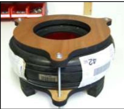
Clean the 2 tyre flanges with thinner to remove residual wax.
