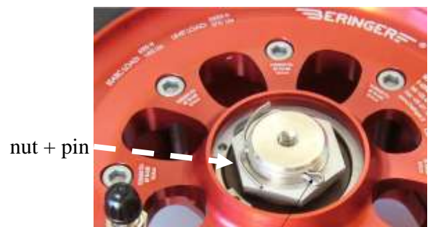
Nylstop slotted nut ou slotted nut + pin
