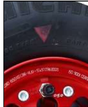
Clean the 2 tyre flanges with thinner to remove residual wax.
