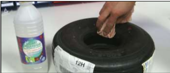
Clean the 2 tyre flanges with thinner to remove residual wax.
